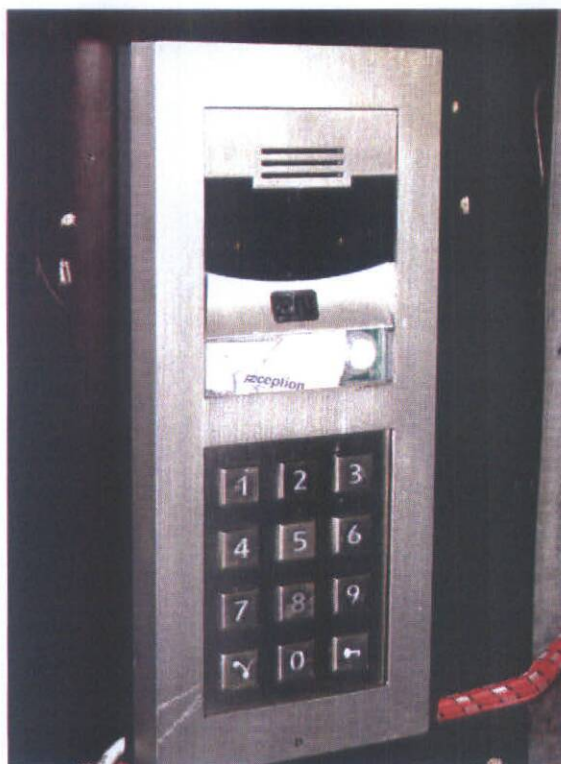
obr. 14 - interkom 2N® Helios IP Verso 9155101C po zkoušce 5
