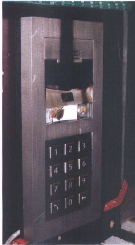
obr. 17 - interkom 2N® Helios IP Verso 9155101C po zkoušce 6
