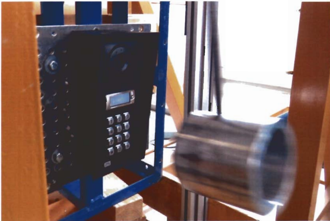
Fig. 12 - IK 10 pendulum hammer test (specimen 2N® Helios IP Force 9151101CK)
