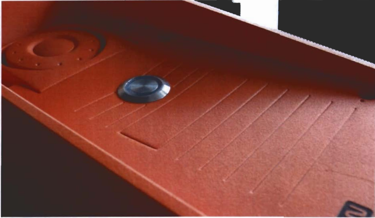
Fig. 15 - enclosure deflection on the specimen 2N® Helios IP Safety 9152101W
