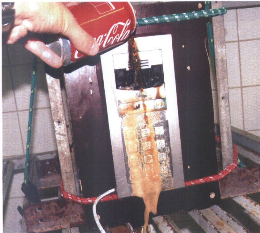
Fig. 18 - test 7 of intercom 2N® Helios IP Verso 9155101C
