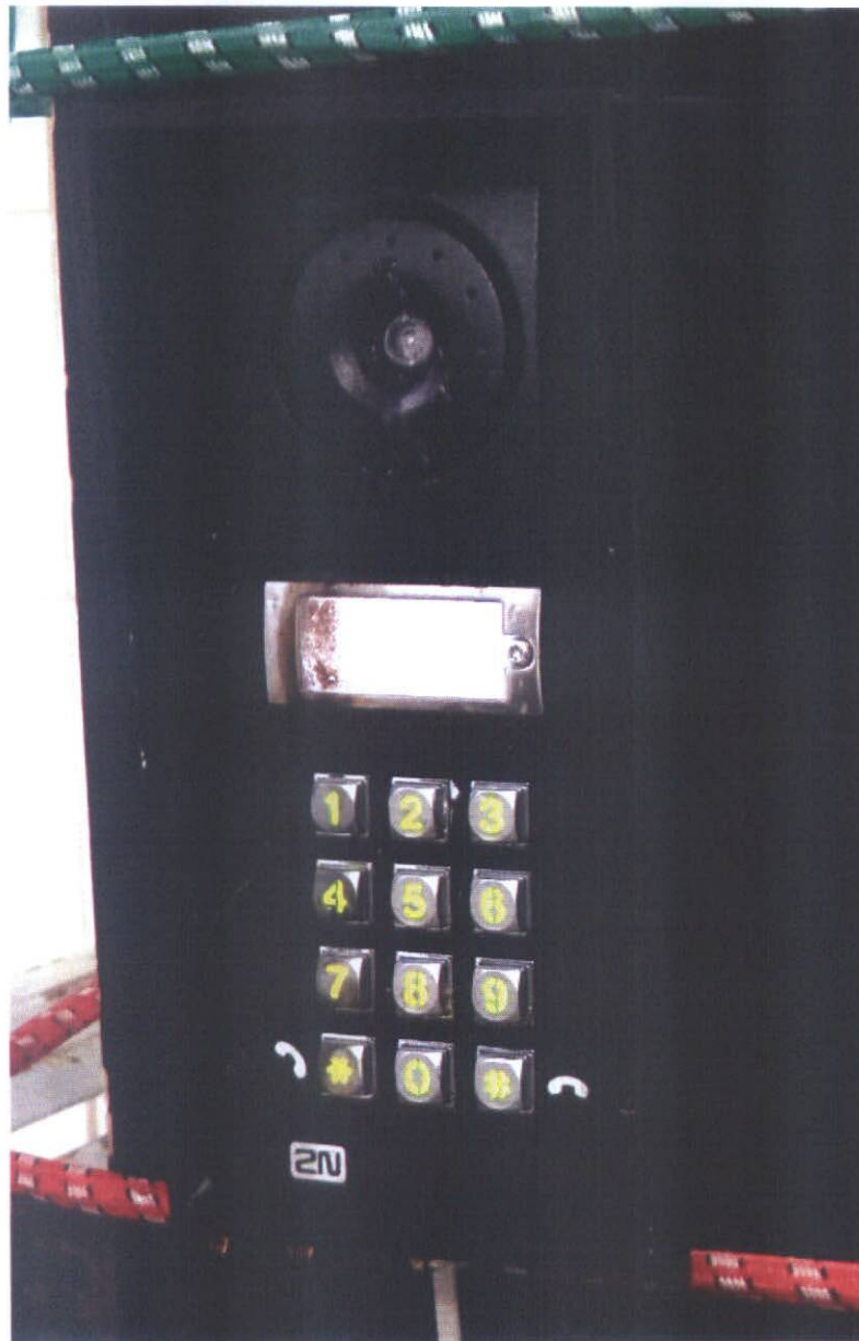
Fig. 11 - functional backlight of all buttons of intercom 2N® Helios IP Force 9151102CRW after testing
