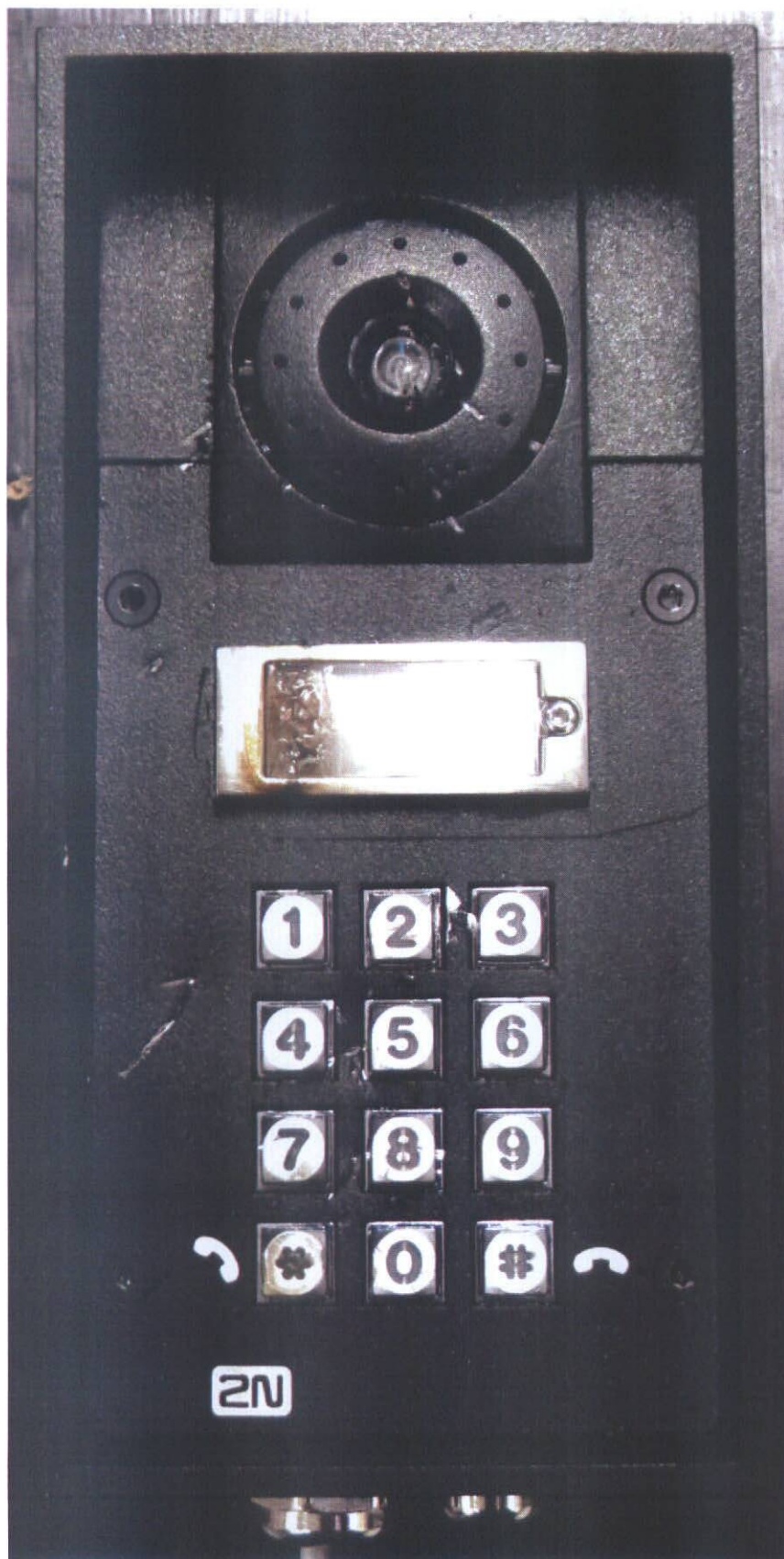
Fig. 12 - intercom 2N® Helios IP Force 9151102CRW after testing
