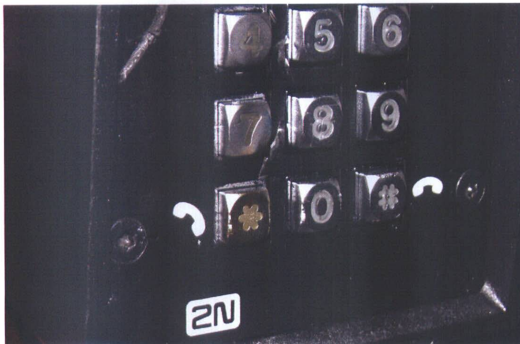
Fig. 10 - button „*“ on the numeric keyboard of intercom 2N® Helios IP Force 9151102CRW after test 6
