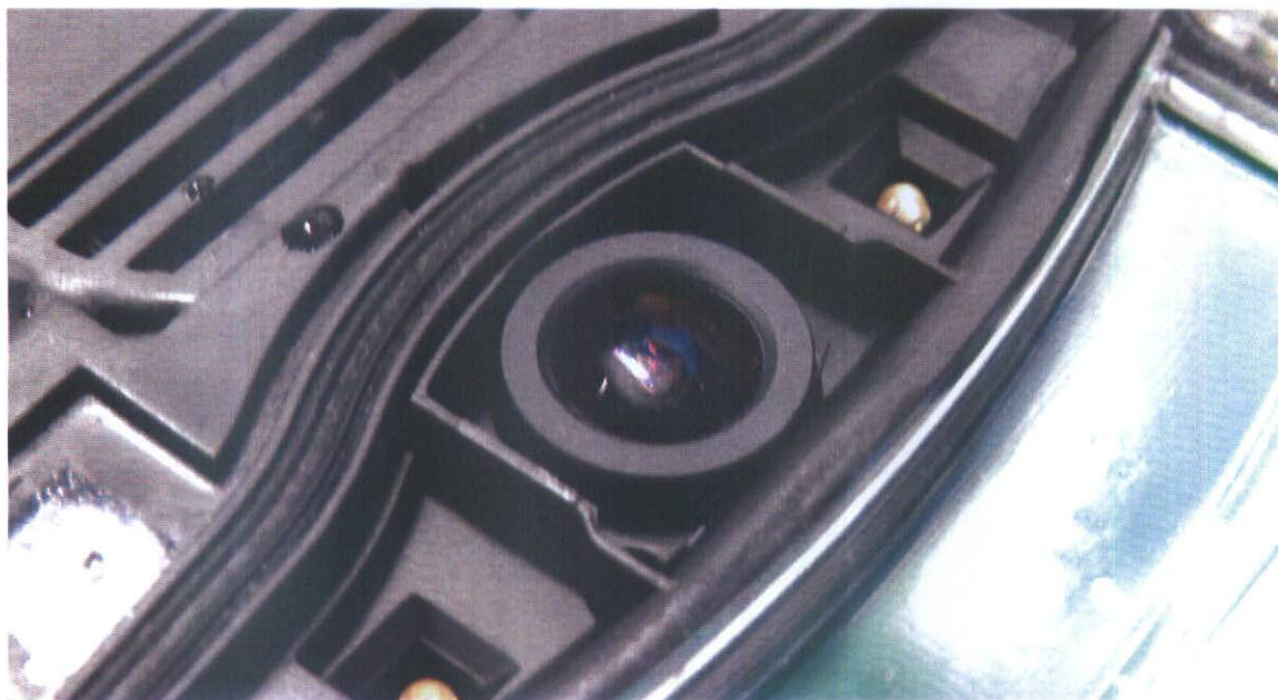
Fig. 22 - undamaged camera of intercom 2N® Helios IP Verso 9155101C
