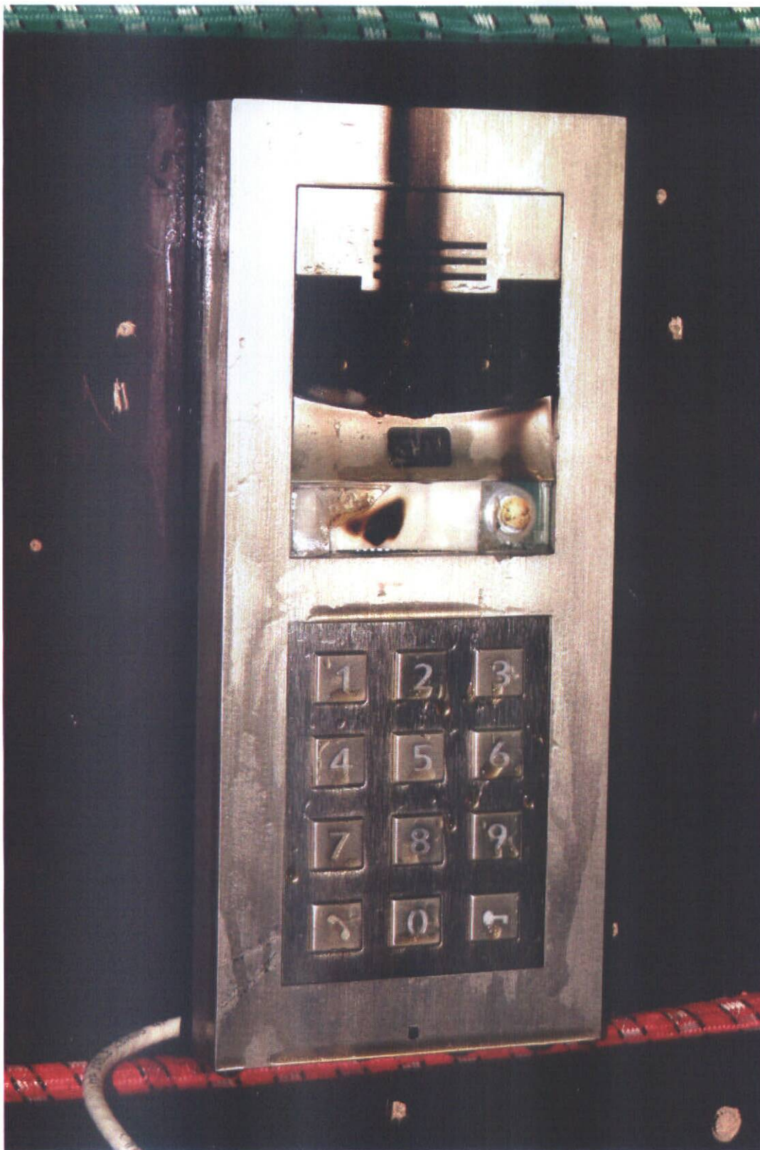
Fig. 19 - intercom 2N® Helios IP Verso 9155101C after testing
