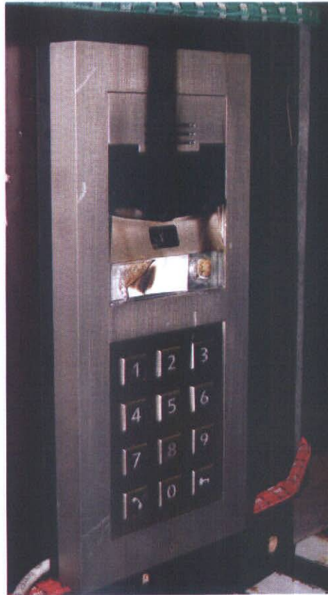
Fig. 17 - intercom 2N® Helios IP Verso 9155101C after test 6
