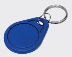
TECHNICAL PARAMETERS Frequency: 125 KHZ Chip: TK4100, FM11RF08 Reading distance: 2~10cm; Material: ABS Working temperature: -10°C to +50 °C Serial numbers: Inkjet Number (various different numbering formats) Size: 41\*33\*4.3mm Colour: blue Weight: 4.5g
