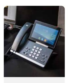
The 24-hour reception desks are equipped with the 2N® IP Phone D7A, a device that receives calls from the entrance intercoms. The 7" touchscreen display shows a preview of the IP intercom cameras and opens the door at the touch of a button.
