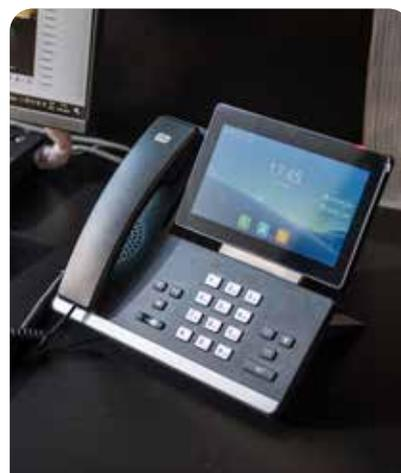
The 24-hour reception desks are equipped with the 2N® IP Phone D7A, a device that receives calls from the entrance intercoms. The 7" touchscreen display shows a preview of the IP intercom cameras and opens the door at the touch of a button.
