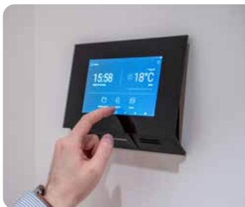
The solution also includes 57 2N® Indoor Touch 2.0 answering units that have been installed in all apartments. This stylish indoor intercom features a sturdy 7" HD tempered glass touchscreen and the option of integration with home automation systems.
