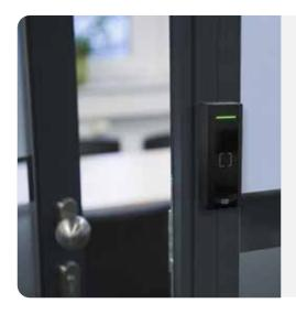
72 2N® Access Unit M RFID access readers were installed at the office doors. These access readers include all the smart hardware directly within them, so the client doesn't have to allocate any space for the controller.
